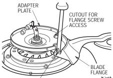
Figure 4 1/4-20 x 11mm PAN HEAD SCREW WITH I OCKWASHER (2)
